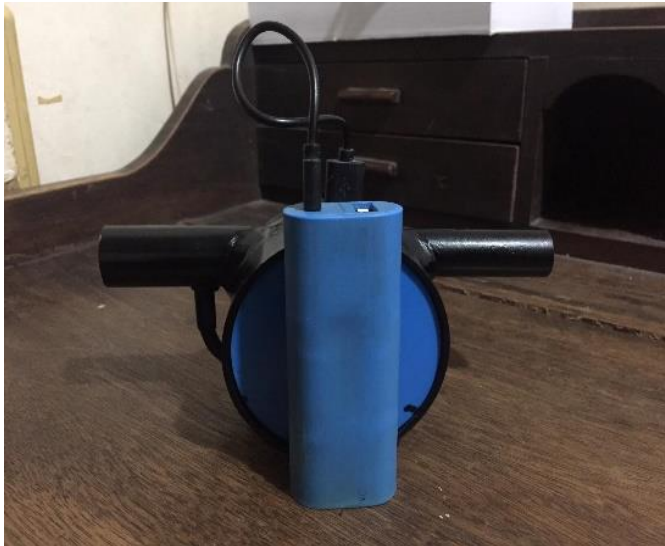
Fig. 3. The Micro-Hydro Generator Turbine.
